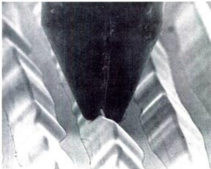
Figure 4. An actual photograph of the Stanton 681 BPD/M bi-pointed stylus tracking the ridge of a stamper. © Stanton Magnetics, Inc. For comparison, a stylus is shown in the groove of a record.
