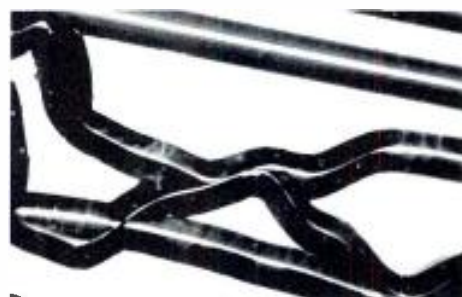
Figure 2. The ultimate test for playback stylus tracking? Not quite—it's just an example of what may happen when the mastering engineer gets some misleading test tones up front.
