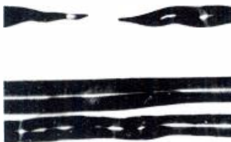
Figure 1. What goes down must come up. Excessive vertical modulation has caused the cutting stylus to lift off, perhaps due to some out-of-phase components in the master tape.
